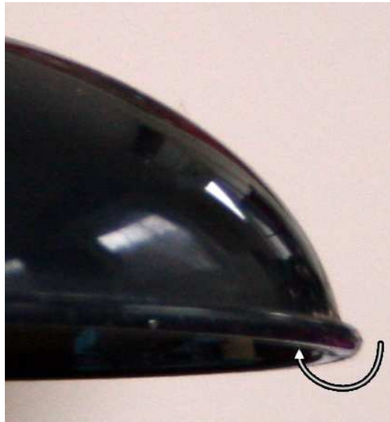
Figure 4.11: Relevance of the teapot effect to our chocolate fountain. The edge of the dome, from which the chocolate falls, is curved, emphasised by the arrow.
