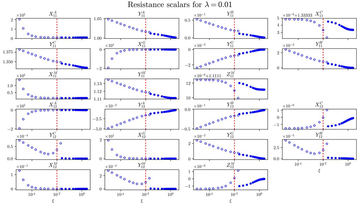
**Figure 3:** Values of the scalar resistance functions over non-dimensional gap,  $\xi$ , for size ratio  $\lambda = 0.01$ . Those generated from the near-field formulae are represented by hollow circles ( $\circ$ ), and those generated from Lamb's solution (Wilson, 2013) are filled circles ( $\bullet$ ). The dashed vertical line appears at  $\xi = \lambda$ , recalling that the near-field formulae are only valid for  $\xi \ll \lambda$ .
