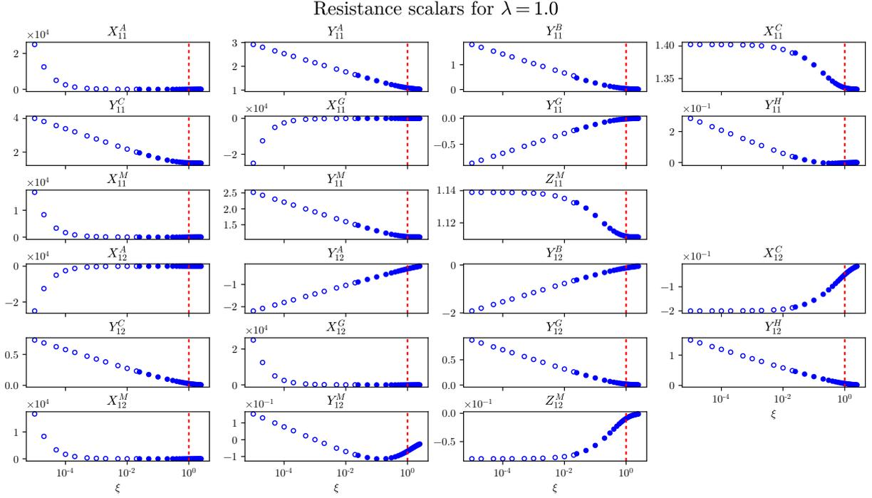
**Figure 1:** Values of the scalar resistance functions over non-dimensional gap,  $\xi$ , for size ratio  $\lambda = 1$ . Those generated from the near-field formulae are represented by hollow circles ( $\circ$ ), and those generated from Lamb's solution (Wilson, 2013) are filled circles ( $\bullet$ ). The dashed vertical line appears at  $\xi = \lambda$ , recalling that the near-field formulae are only valid for  $\xi \ll \lambda$ .
