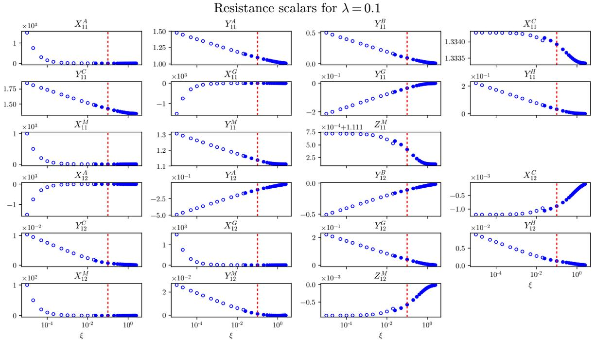
**Figure 2:** Values of the scalar resistance functions over non-dimensional gap,  $\xi$ , for size ratio  $\lambda = 0.1$ . Those generated from the near-field formulae are represented by hollow circles ( $\circ$ ), and those generated from Lamb's solution (Wilson, 2013) are filled circles ( $\bullet$ ). The dashed vertical line appears at  $\xi = \lambda$ , recalling that the near-field formulae are only valid for  $\xi \ll \lambda$ .
